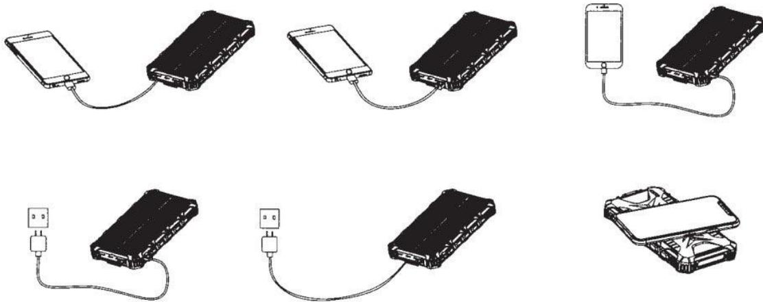
To recharge the power bank via the solar panel, please put the power bank in direct sunlight and make sure the solar panel is positioned towards the sun. The solar charging indicator will turn green while the charging is in process, and turn blue when the power bank is fully charged.
