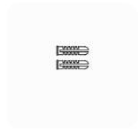
Two expansion anchors
