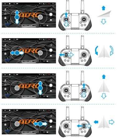
Push the left joystick up, and the main blade speed increases and the drone rises. Push the left joystick down and the drone lowers down.
