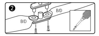
Unscrew the bolt to separate the two blades and replace them. Replace the damaged D/B labeled blade with the new D/B labeled blade and the damaged A/C with the new A/C blade.
